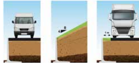
DLF10GSZ uniform distributed overload 25 kN/m 2
