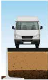
DLF10GSZ uniform distributed overload 25 kN/m 2
