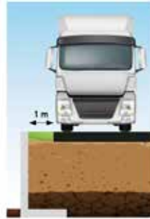
DLF10GS uniformly distributed overload 40 kN/m 2 at edge distance 1 m equivalent to load mode LM1 according to NBN EN 1991-2
