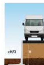
DLF10GSRZ uniform distributed overload 25 kN/m 2
