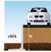
CLF10GSRZ uniform distributed overload 10 kN/m 2 light traffic max. 3.5 tons
