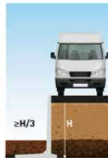
DLF10GSRZ uniform distributed overload 25 kN/m 2
