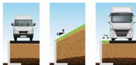
DLF10GS uniform distributed overload 25 kN/m 2
