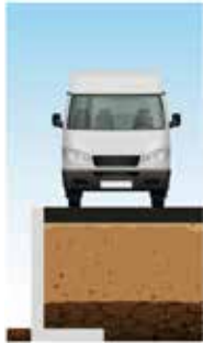
DLF10GS uniform distributed overload 25 kN/m 2
