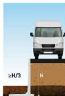
DLF10GSRZ charges standard 25 kN/m 2
